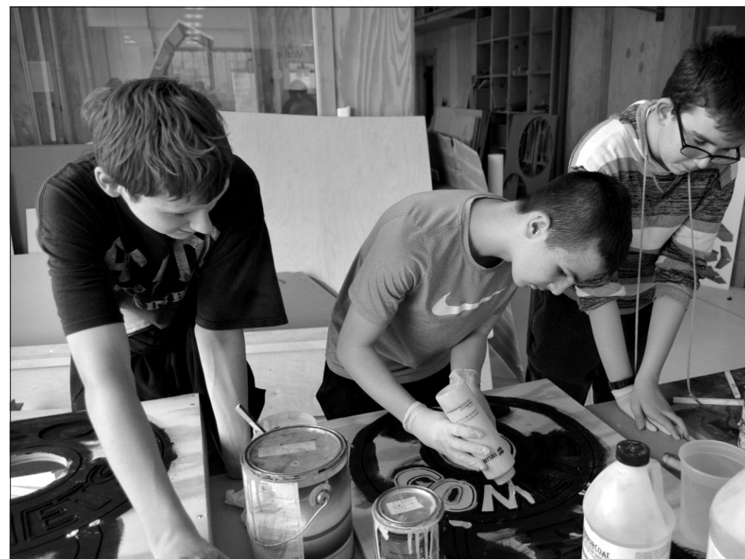
Fallsburg students pour colored resin into the routed drawings on the boards.
