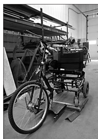
A bicycle is being modified at THINC so it will fit any wheelchair.
